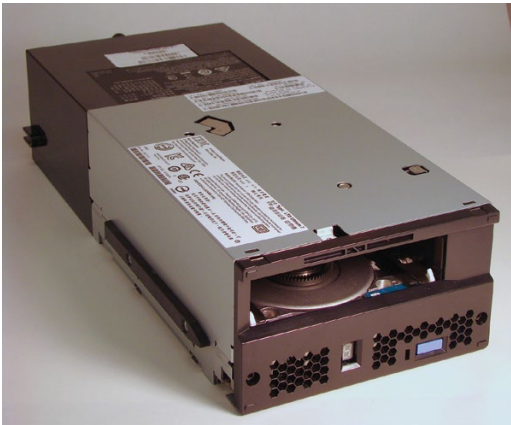
Figure 5. The LTO Ultrium 7 drive that goes into IBM TS4500 Tape Library.
