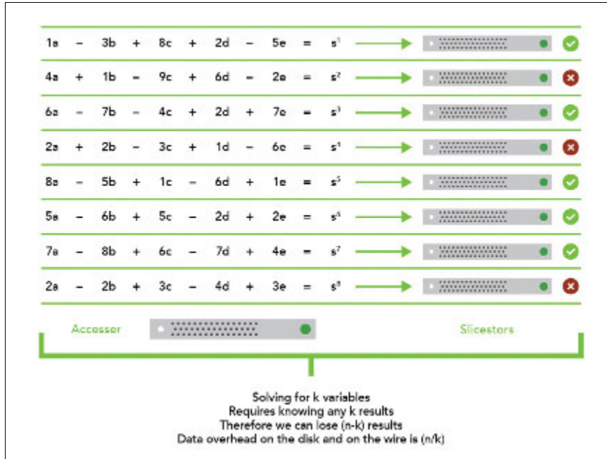
Figure 4-28 Example of calculations to illustrate how information dispersal works
